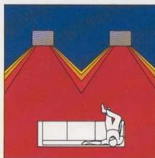
Model 14's constant directivity MANTARAY™ keeps dispersion angle constant for all frequencies.
