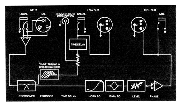
ELECTRONIC DIVIDING NETWORK BLOCK DIAGRAM
